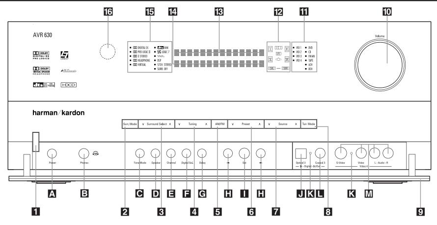
The following controls and indicators are available on the AVR 630's front panel:
